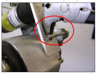
Inspect the plate bushing for wear. Replace it if it is worn or uneven.
