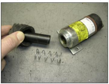
Check that the catch arm engages the clutch collar when the solenoid is energized. The solenoid plunger should retract completely and the catch arm should contact the aluminum stop collar squarely.
