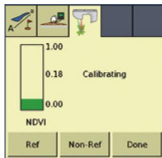
The GreenSeeker plugin tab now includes **Ref** and **Non-Ref** buttons, along with a NDVI bar graph showing the real-time combined average NDVI from the RT200 module.
