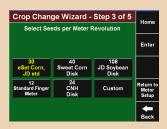
**Step Three:** Select your metering system. If you have a metering system with a seeds per meter revolution that is different than the options listed, you can set a custom number under the 'Custom' button.
